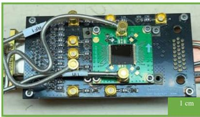
Wired sample before cryogenic cooling
